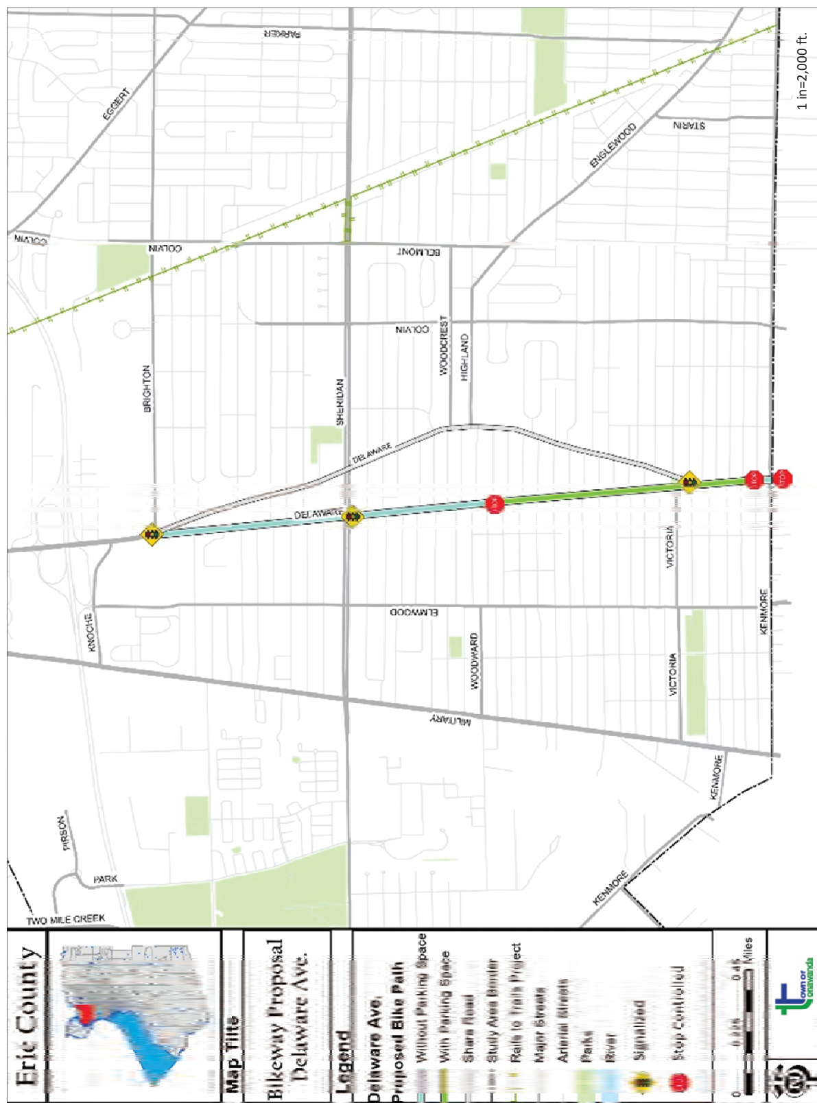
Figure 4.17 Map of proposed bike path and intersection treatment facilities.
